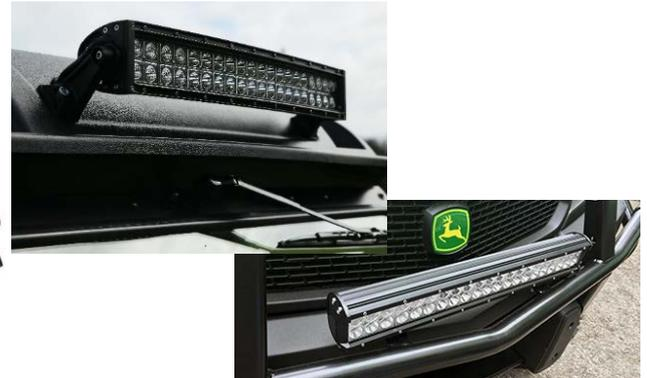
Upgrade your lighting with a new range of supplementary LED work lights from Vapormatic. These versatile lights are compatible with all types of vehicle – from utility and harvesting vehicles to all makes of tractor – available in 335mm single bolt, 543mm curved, 502mm, 615mm and 865mm straight models.
