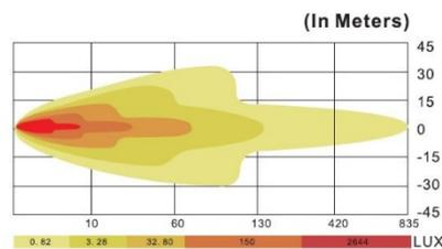
Dual-row 543mm wide LED design with 40 CREE LEDs delivers 8,800 lumens (raw) of cool white light. Curved profile also ensures wider light dispersal and illuminates everything in and around the forward path of the vehicle. Powerful combo spot/flood light beam simultaneously provides long distance terrain and field illumination. IP67 approved – dust tight and protected from water immersion up to 1m for 30mins. 12-24V operation. ECE R10 approved
