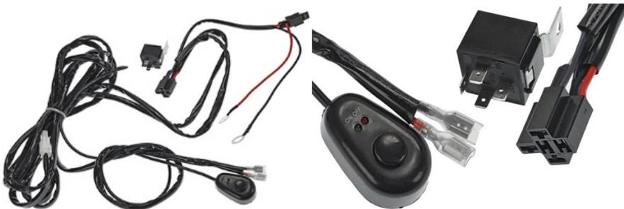
Plug and play wire harness for universal lighting. Complete with on/off switch and LED indicator, allowing you to easily control the lighting from the comfort of your cab. Also includes; 30 Amp fuse, and 42 Amp automotive relay with solderless spade connections. Cable length 3000mm.
