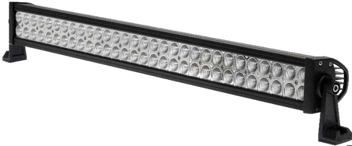
Larger, 865mm bar width combined with a 60° flood light beam gives greater distance to your night vision and excellent illumination in and around the forward path of the vehicle. Dual-row design with 60 powerful LED's delivers an impressive 16,200 lumens (raw) of cool 6000K white light. IP67 approved – dust tight and protected from water immersion up to 1m for 30mins. 12-24V operation. ECE R10 approved.
